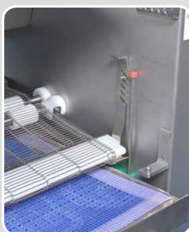
Lye Liquor level indicator No lye stone, that prevents sight; no extra leakage risk.
